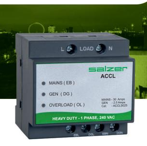
When Mains supply fails and Generator supply starts, ACCL transfers the load from Mains supply to Generator automatically. It also acts as a current limiter when load on generator exceeds the preset limit, thus avoiding any overload on the generator.
